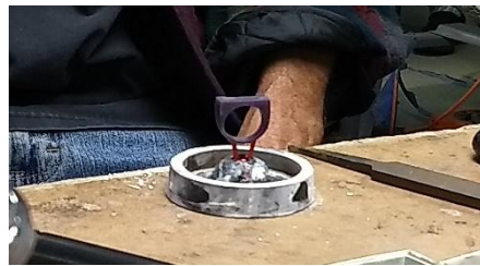
Placing sprues on a formed model
